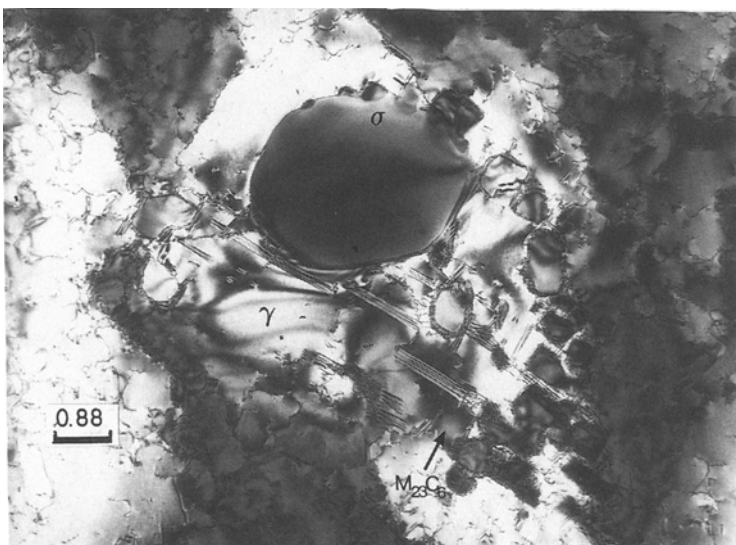
Figure 12 TEM micrograph showing small amounts of intermetallic phase in 304W after 3000 h at 700^\circ\text{C} .
